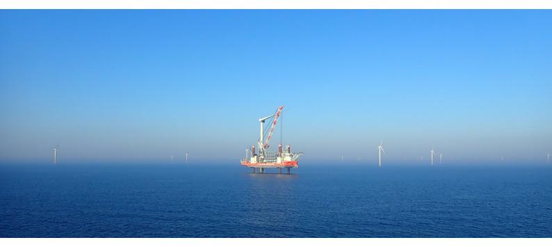
25 September 2019, installation vessel Bold Tern installed the last of 91 turbines on Hornsea One offshore wind farm. The complete wind farm consists of a total of 174 Siemens Gamesa SWT-7.0-154 turbines and is the world's largest offshore wind farm to date.
